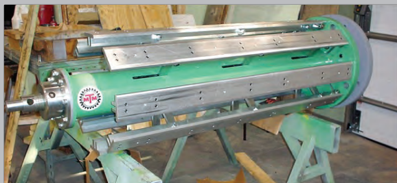
Fig. 13 Rectangular and Round Expanding Mandrels
