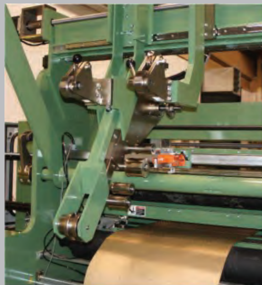
Fig. 11. Wire Flatteners added to an existing machine
