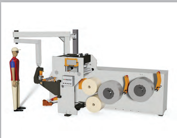
In last generation winding machines, operator faces front to the coil being wound. Insulation, foils and wires are fed from the back of the machine
