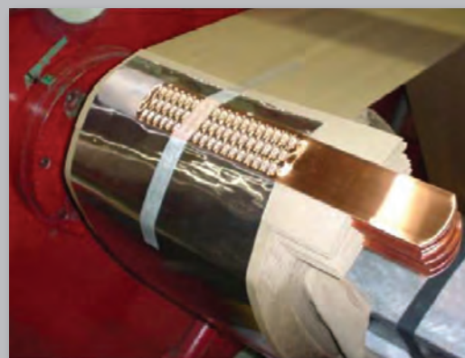
Fig. 12. Integrated Cold Welding System for Coil Terminals Distribution and Small Power Transformers
