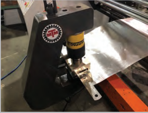
Fig. 12A. Portable Cold-Welding Unit for Coil Terminals Distribution and Small Power Transformers
